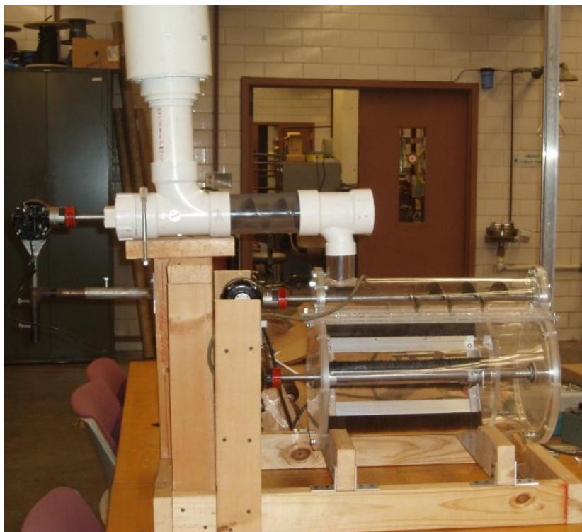
Figure 6-9. Acrylic prototype of double-shaft ketone reactor.
