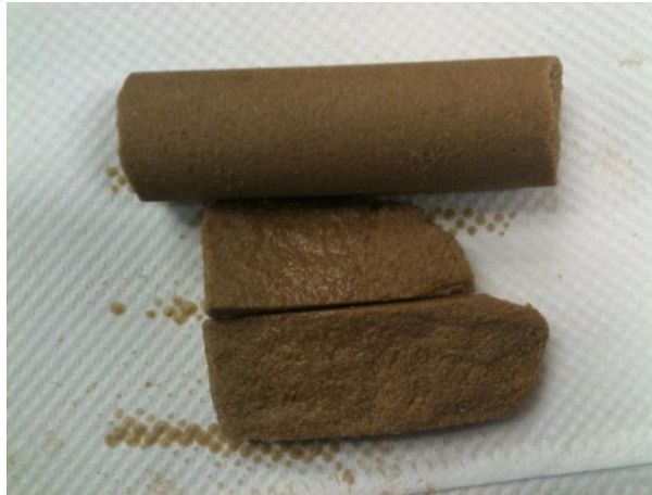
Fig. 3.28— Bentheimer sandstone core right after emulsion flow experiment.
