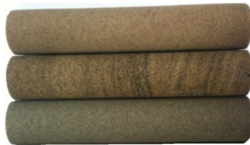
Fig 3 12— Bentheimer sandstone, Idaho sandstone and Boise sandstone from top to bottom of size 1
