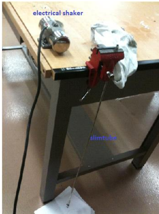
Fig. 2.4— Setup for packing a slimtube with sand.
