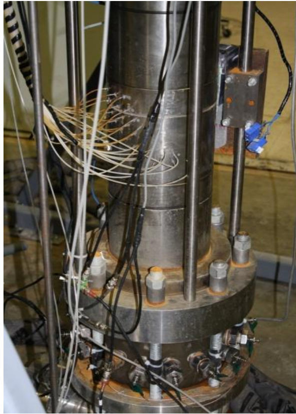
Figure 13. MVP with instrumentation installed
