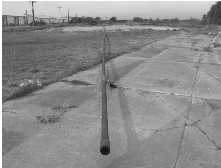
Figure 4.1: Photograph of the 2-7/8" pipe string - no concrete case
