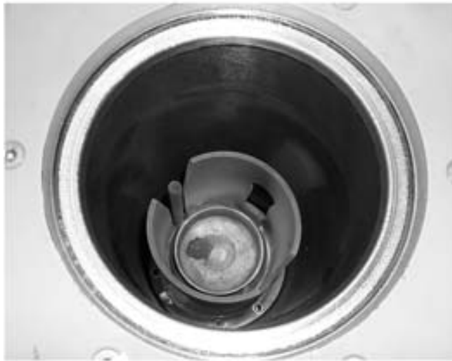
Fig. 13. QIH-3 Mini-hipper and detail of furnace.
