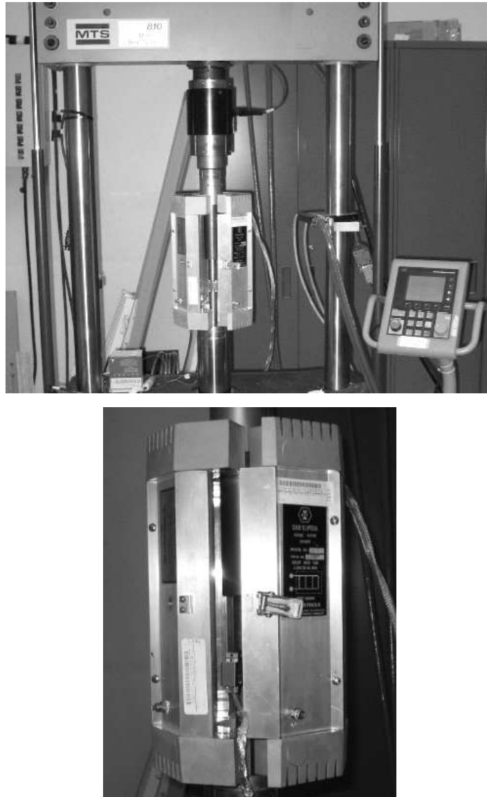
Fig. 26. MTS test system showing furnace and testing fixture.
