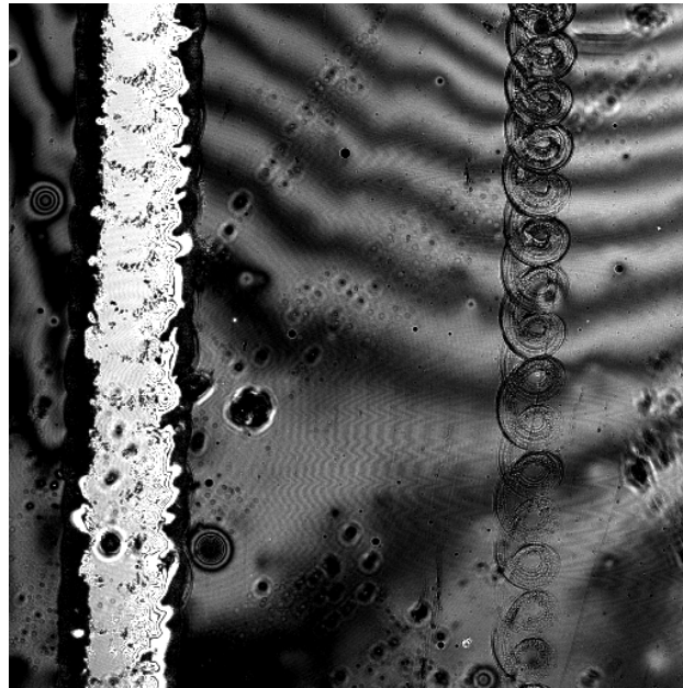
Figure 4.10. Wake of tool (right) while machining line on PMMA. Image shows the machining of lines is continuously creating hole like structures. Local surface irregularity makes machining beyond the PMMA layer (left).
