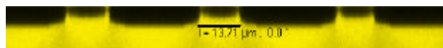
Figure 3.10. Etch profile of corning 0211 glass with chrome as etch mask and intermittent acid wash. Total gas flow rate of 16 sccm in CF 4 :O 2 at 14:2 flow ratio. Glass etched at P=200W for 15 minutes. Intermittent wash with 1M HCl and 15 seconds of HF etch after every 5 minutes. Cycle repeated 3 times. Confocal image is up side down.
