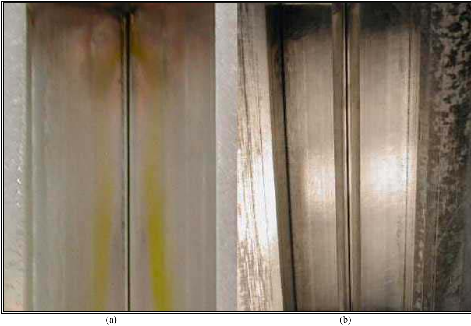
Figure 27. Comparison of particle deposition on LSVI Unit 6 receiver nozzle WITHOUT secondary expansion (a) and LSVI Unit 7 receiver nozzle WITH secondary expansion (b) for monodisperse liquid aerosol particles tagged with fluorescent tracer.
