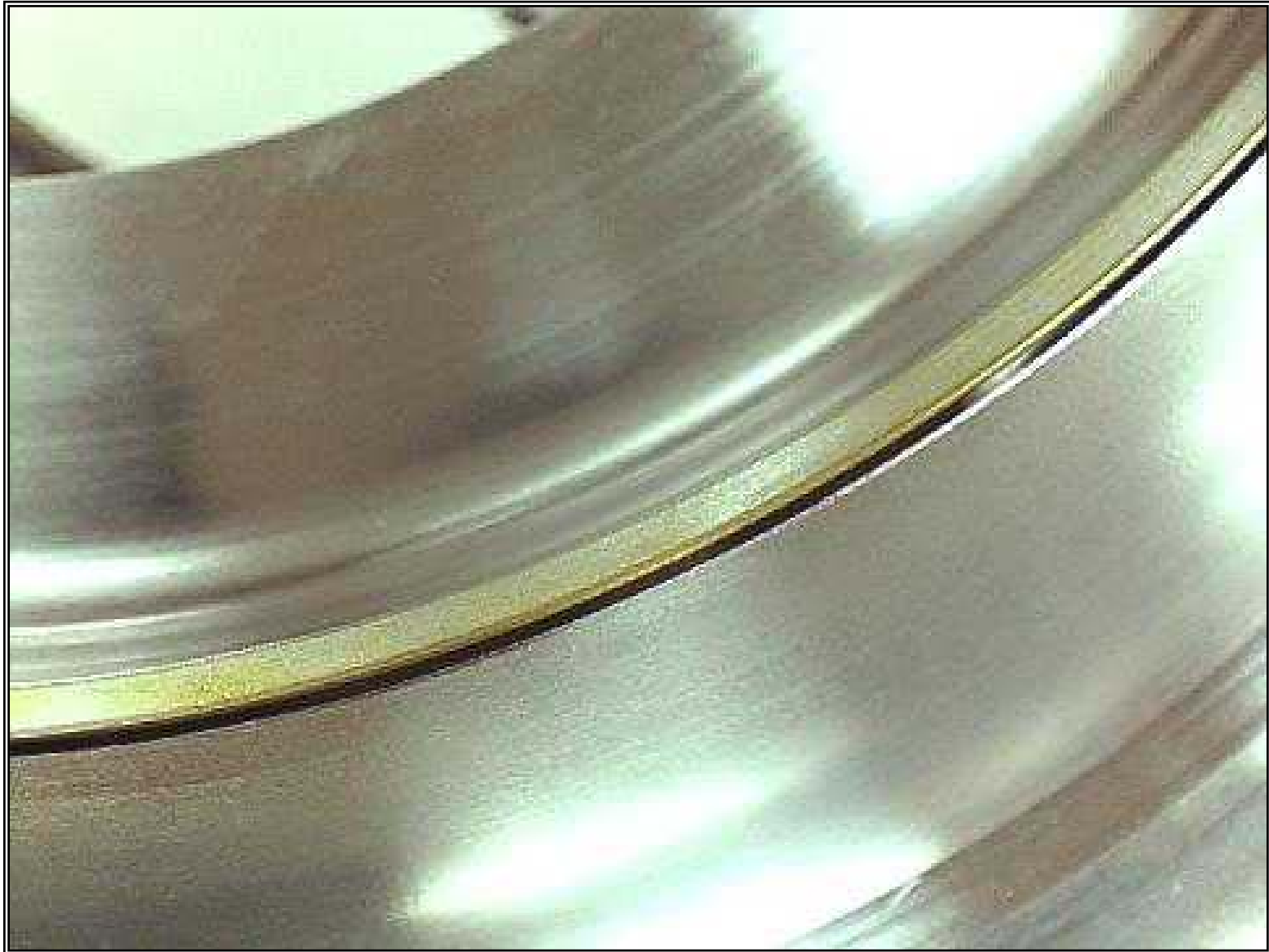
Figure 29. Deposition of 6.6 \mu\text{m} AD monodisperse liquid aerosol particles on the receiver nozzle throat in CSVI Unit 1.
