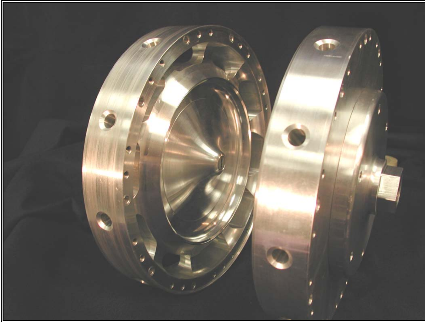
Figure 6. Photograph of prototype CSVI unit (split into half-assemblies).
