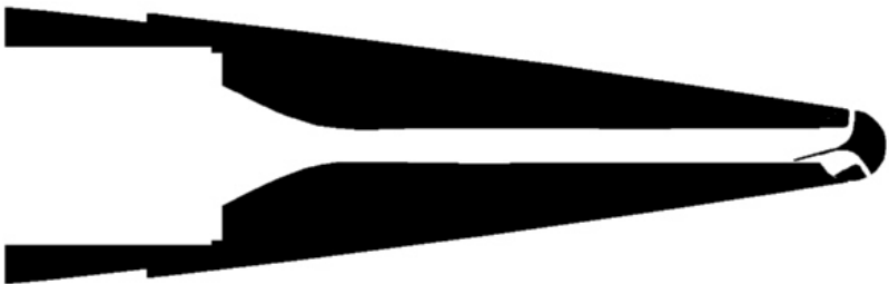
Figure 4.3 Cross Section of Trailing Edge Showing Narrow Plenum Design
