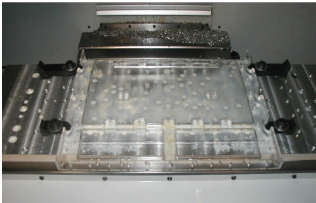
Figure 3.5. Upper Wing Panel of the Leading Edge Model
