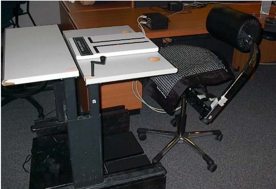
Figure 15. Experimental Set-Up and Xsensor Pressure Pad.
