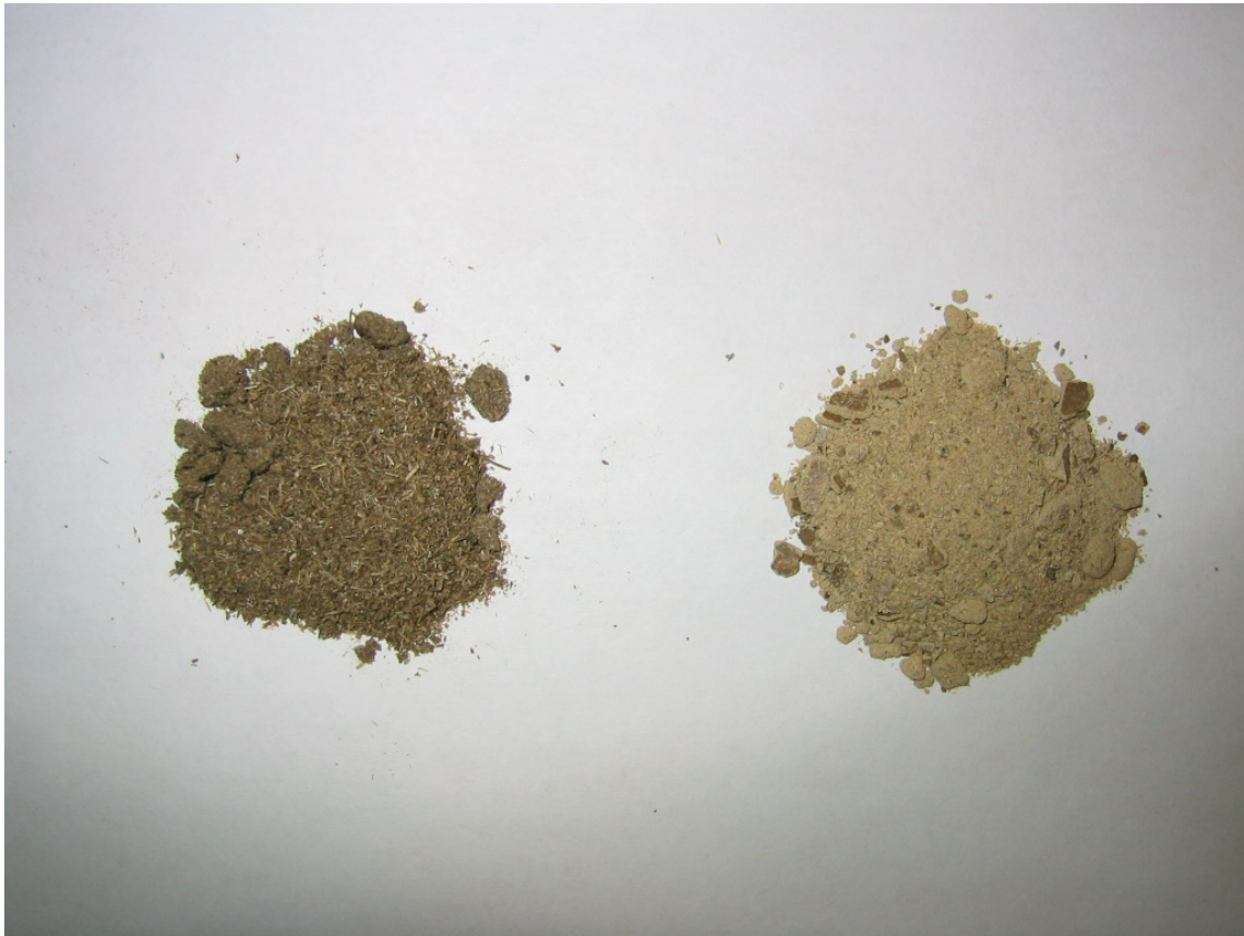
Figure 4.86 Photograph of old bagasse after 6 months of lime treatment at 50°C under non-oxidative (left) and oxidative (right) conditions.
