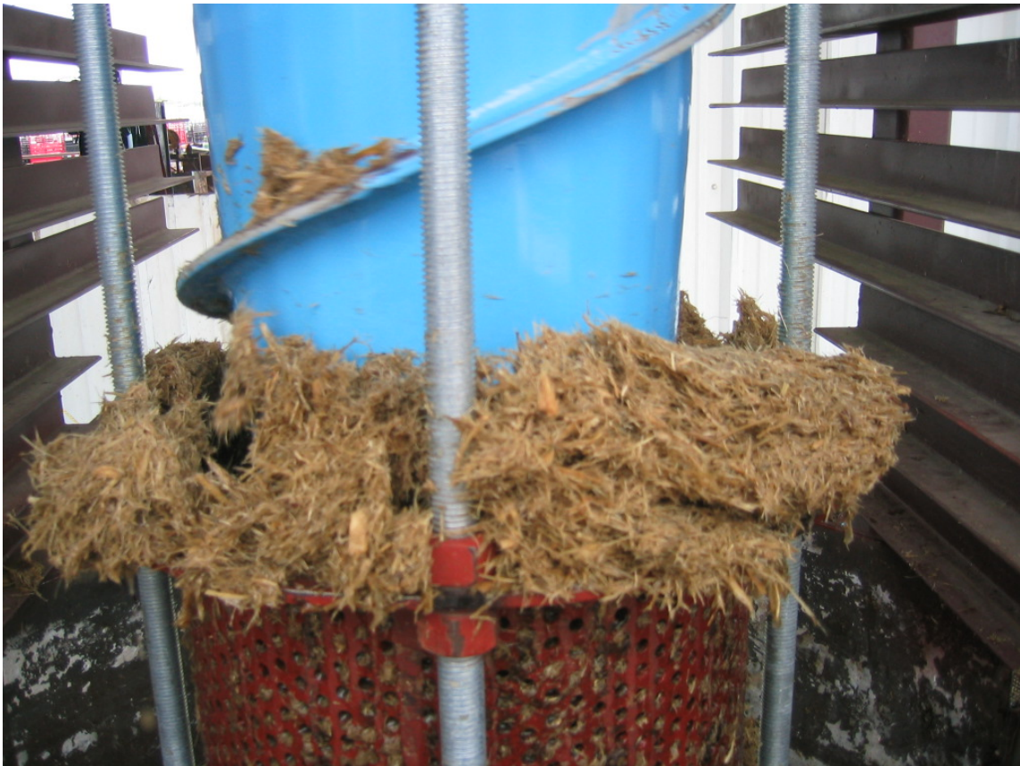
Figure 2.13 Photograph of the screw-press conveyor during operation.
