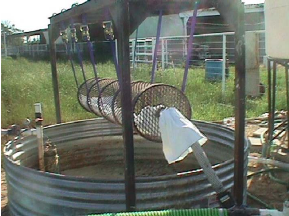
Figure 3.25 Photograph of one of the filters (i.e., cloth and cage) after assembly.
