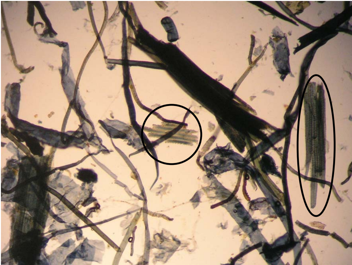
Figure 4.85 Digital micro-photograph of the bagasse pulp from Batch #2 showing some pith particles (circled).
