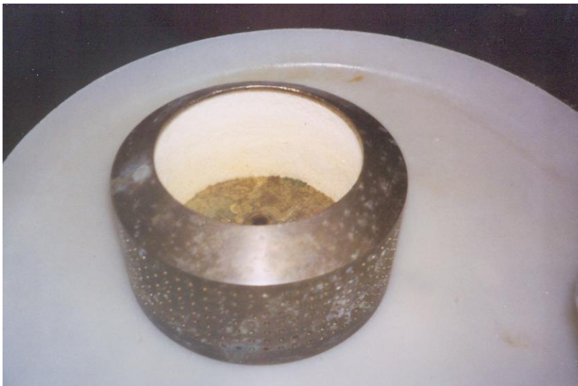
Figure 3.31 Photograph of centrifuge basket showing the crystals from preserved juice crystallization attached to its interior (Audubon Sugar Institute).
