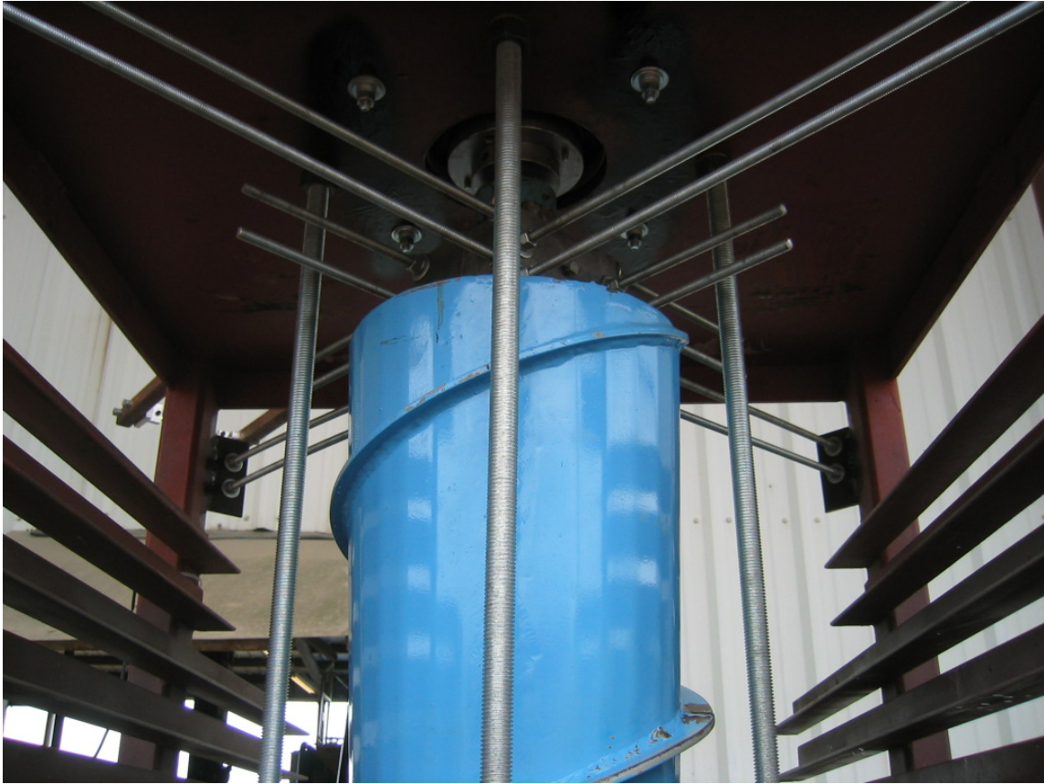
Figure 2.11 Photograph showing details of the screw-press conveyor flight, the tray holder/rails for the collecting trays, and the shaft support.
