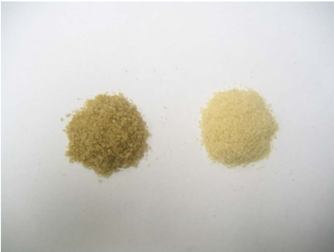
Figure 3.38 Photograph of conventional mill raw sugar, ICUMSA 2770 (left) and sugar from preserved juice, ICUMSA 1820 (right).
