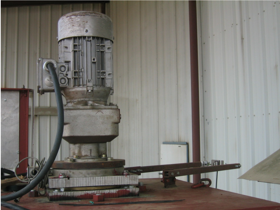
Figure 2.10 Photograph of the motor and torque-measuring system.
