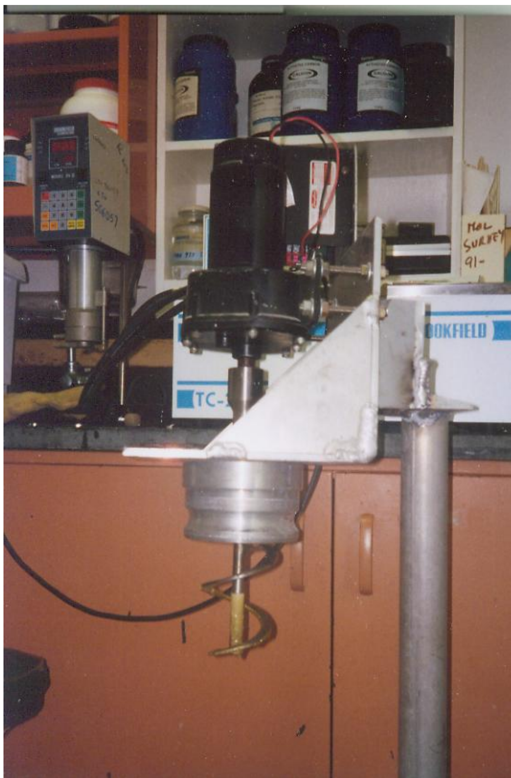
Figure 3.29 Internal details of the bench-scale crystallizer (Audubon Sugar Institute).
