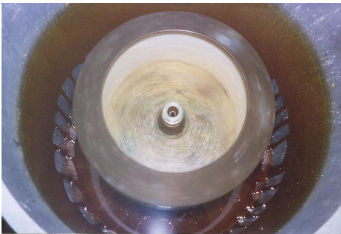
Figure 3.30 Photograph of the separation by centrifugation of sugar crystals from molasses in massecuite from preserved juice (Audubon Sugar Institute).
