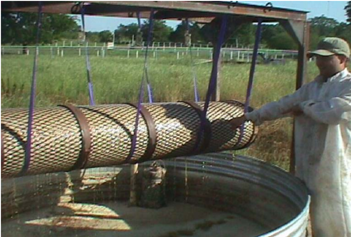
Figure 3.26 Photograph of the pilot scale filtration taking place (only one filter being used).
