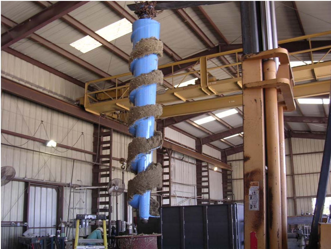
Figure 2.21 Photograph of the screw-press after operation being pulled out of the perforated outer casing.
