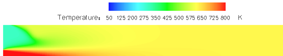
Fig. 32. Converged results for coarse grid with \dot{m} = 1.127 \text{ kg/s} LN_2 injection.
