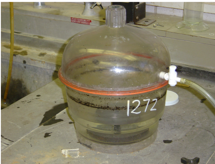
Figure 7.6. Vacuum Apparatus for Wet Conditioned Specimens.
