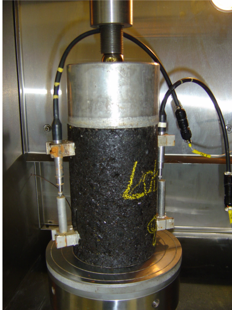
Figure 7.8. Dynamic Creep Test Set Up with Axial LVDT.
