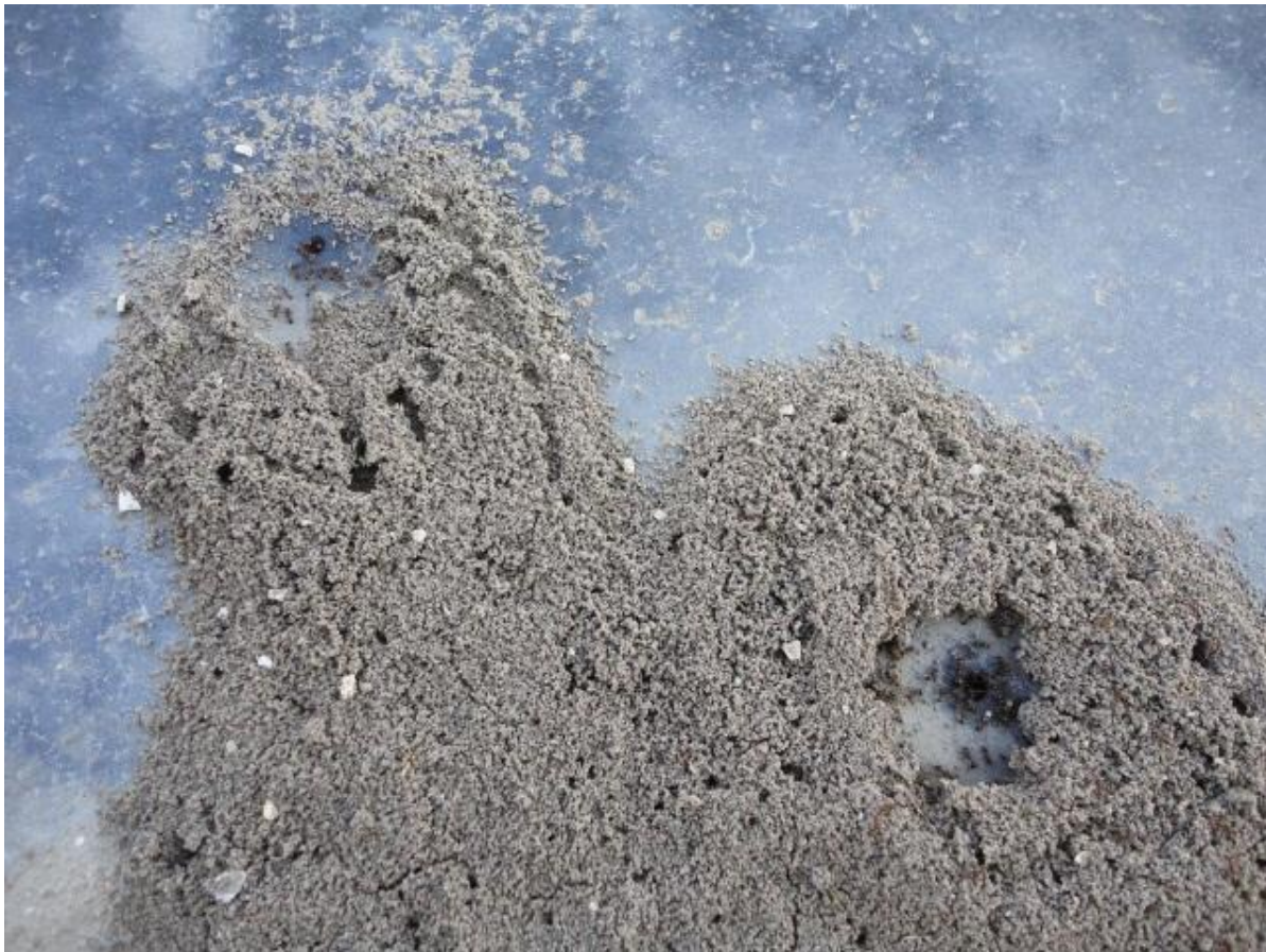
Figure 10. Ant colony in the EPDM rubber liner
