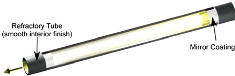
Fig. 9. Hollow-Core Light Guide Concept.
