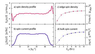
FIG. 1. (Color online) Spin Hall effect in a 2DHG. Spatial profile of the z component of spin (a), and of the spin current (b) across the channel width (x direction). Disorder dependence of the accumulated edge-spin density (c), and of bulk spin current (d).
