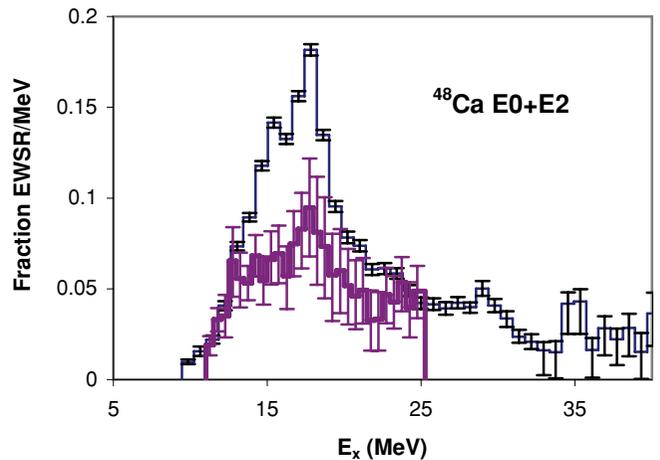
FIG. 7. (Color online) The  $E0 + E2$  strength distribution obtained in this work for  $^{48}\text{Ca}$  is shown in the histogram with thin lines. The darker histogram is the  $E0 + E2$  strength distribution obtained from inelastic electron scattering [16]. The vertical scale indicates the fraction of the  $E0 + E2$  sum rule observed.
