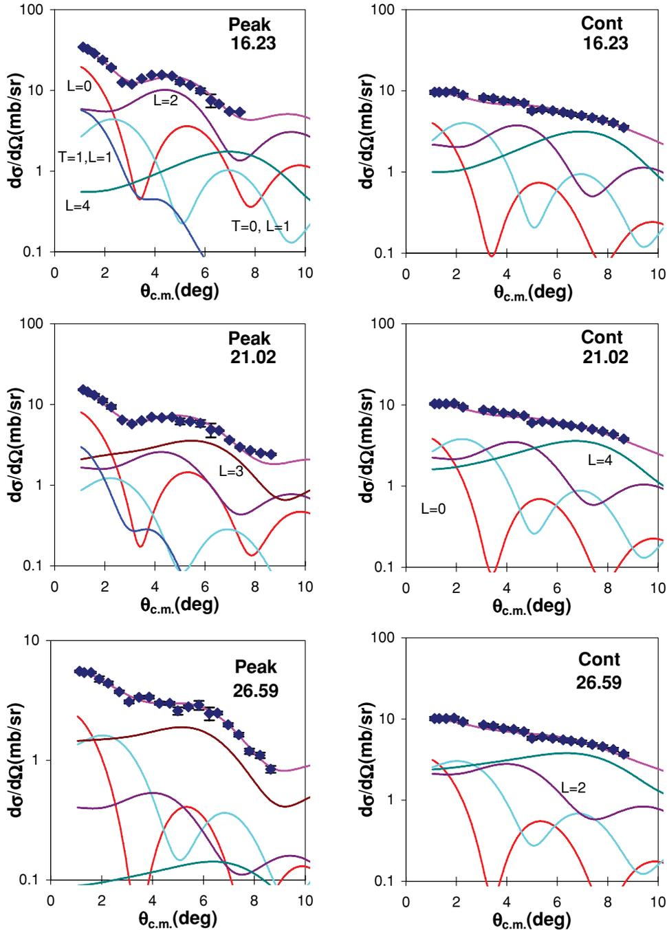
FIG. 4. (Color online) The angular distributions of the  $^{48}\text{Ca}$  cross section for three energy bins of the GR peak and the continuum. The excitation energy in MeV of the center of the bin is shown. The lines through the data points indicated the multipole fits. Contributions of each multipole are shown.
