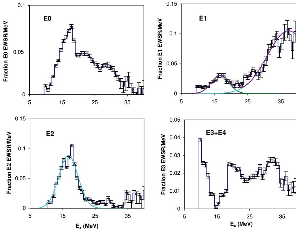
FIG. 5. (Color online) Isoscalar strength distributions obtained for  $^{48}\text{Ca}$  are shown by the histograms. Error bars represent the uncertainty from the fitting of the angular distributions and different choices of the continuum, as described in the text. Gaussian fits are shown as smooth lines. The vertical scale on the  $E3 + E4$  distribution is in terms of the  $E3$  EWSR only.
