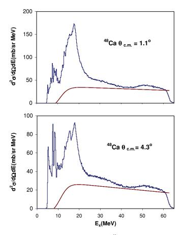
FIG. 1. Inelastic  $\alpha$  spectra obtained for <sup>48</sup>Ca. The solid lines show the continuum chosen for the analysis.
