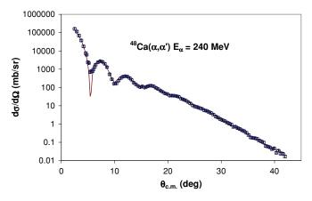
FIG. 2. (Color online) Angular distribution of the differential cross section for elastic scattering for 240-MeV  $\alpha$  particles from <sup>48</sup>Ca plotted vs c.m. angle. The error bars include uncertainty from statistical as well as systematic error. The solid line shows an optical model calculation with the parameters listed in Table I.
