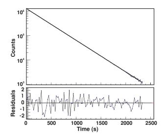
FIG. 1. (Color online) The decay of <sup>198</sup>Au in gold (III) oxide, at room temperature. Experimental data appear as dots in the upper portion of the figure; the straight line is the fit to these data. Normalized residuals are shown at the bottom.
