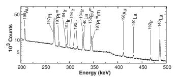
FIG. 4. Portion of the  $\gamma$ -ray energy spectrum measured 6 h after the spectrum shown in Fig. 3. Peaks are identified by their  $\beta$ -decay parent except for the 346.5-keV peak, which is due to the isomeric transition from <sup>197</sup>Pt<sup>m</sup>.
