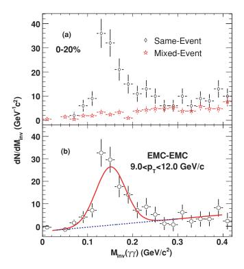
FIG. 2. (Color online) The diphoton invariant mass distributions using the EMC-EMC method in 0–20% Au + Au collisions at  $\sqrt{s_{NN}} = 200\,\text{GeV}$ . The solid line is a fit result of a Gaussian peak plus a background function. The residual background is shown as a dotted line. Panels (b) is the distribution after mixed-event background subtraction from panel (a).
