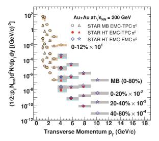
FIG. 6. (Color online) Invariant yield of STAR  $\pi^0$  as a function of  $p_T$  at midrapidity for different collision centrality bins in Au + Au collisions at  $\sqrt{s_{NN}} = 200 \, \text{GeV}$ . Spectra for different collision centralities are scaled for clarity. Statistical errors are shown as vertical lines and point-to-point systematic errors are shown as bars.
