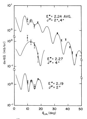
FIG. 5. <sup>138</sup>Ba( $\alpha$ ,  $\alpha'$ ) angular distributions showing separate components of a doublet at 2.24-MeV average energy.
