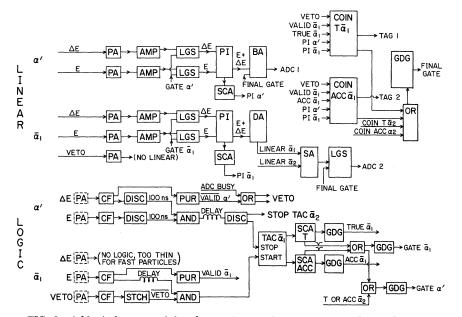
FIG. 2. A block diagram of the electronics. Only one decay stack is indicated.
