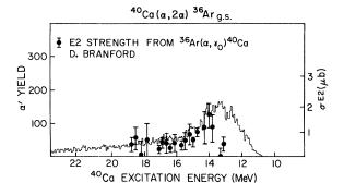
FIG. 14. Projection of  ${}^{40}\text{Ca}(\alpha, 2\alpha){}^{36}\text{Ar}(\text{g.s.})$  events onto the  $\alpha'$  axis [Fig. 4(c)] which has been labeled on a  ${}^{40}\text{Ca}$ excitation energy scale. These events were measured with the  $\overline{\alpha}$  detector at  $\theta = -120^{\circ}$ . Also plotted are E2 cross sections deduced from  ${}^{36}\text{Ar}(\alpha, \gamma_0){}^{40}\text{Ca}$  measurements of Branford (Ref. 8).
