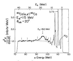
FIG. 3. A  ${}^{40}Ca(\alpha, \alpha'){}^{40}Ca$  spectrum taken at 20°. The dashed line indicates the empirically determined shape of continuum underlying the GQR.
