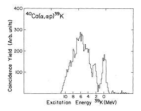
FIG. 5. True coincident events from the  ${}^{40}$ Ca( $\alpha$ ,  $\alpha' p$ ) ${}^{39}$ K reaction projected onto an axis perpendicular to kinematic loci corresponding to population of states in  ${}^{39}$ K [Fig. 4(e)]. Only those events whose  $\alpha'$  energy would correspond to excitation of  ${}^{40}$ Ca into the GQR region (16.4  $\leq E_x \leq 20.7$  MeV) are included.
