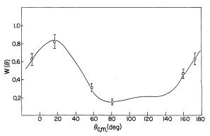
FIG. 13. Angular correlation function for  $\alpha$  decay of the 13.9-MeV state in <sup>40</sup>Ca to the ground state of <sup>36</sup>Ar. The errors shown include an estimate of the uncertainty in extracting the peak yield. The solid curve is a theoretical calculation for decay of a  $J^{\pi} = 2^+$  state performed as described in the text.
