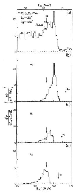
FIG. 12. Decomposition of the  ${}^{40}Ca(\alpha, 2\alpha)$  coincidence spectrum projected onto the  $E_{\alpha'}$  axis. The total true yield is shown in (a). The projection of events leaving  ${}^{36}Ar$  in its ground state (b), first-excited state (c), and in states around  $E_x = 4$  MeV (d) are also shown. These projections are the type in [Fig. 4(c)]. The GQR position, *n* threshold, and  $\alpha$  decay thresholds are indicated.
