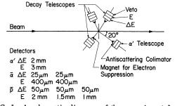
FIG. 1. A schematic diagram of the experimental geometry. The decay telescopes were mounted on a single turntable which rotated relative to the  $\alpha'$  detector.
