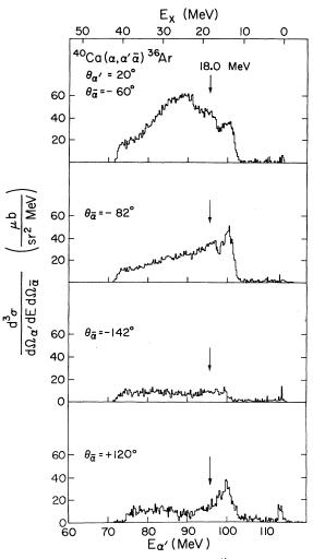
FIG. 11. Projections of the total true  ${}^{40}Ca(\alpha, 2\alpha)$  coincidence spectra measured at several angles onto the  $\alpha'$  axis [Fig. 4(a)]. The top spectrum was measured near the quasifree angle and shows a large knockout contribution. The arrow indicates the position of the GQR.
