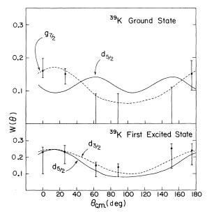
FIG. 9. Angular correlation functions for proton decay of the GQR. The curves are the result of DWBA calculations and the experimental points are the values extracted from the coincidence measurement. The angle is with respect to the  $^{40}$ Ca recoil direction. The proton partial waves are indicated.
