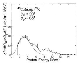
FIG. 7. A spectrum of protons in coincidence with  $\alpha$  particles whose energy corresponds to excitation of <sup>40</sup>Ca between 16.4–20.7 MeV. The proton energy is given in the <sup>39</sup>K + *p* center of mass system. The dashed curve represents a simple estimate of the shape of the spectrum from level density and penetrability considerations and has been arbitrarily normalized to the data.
