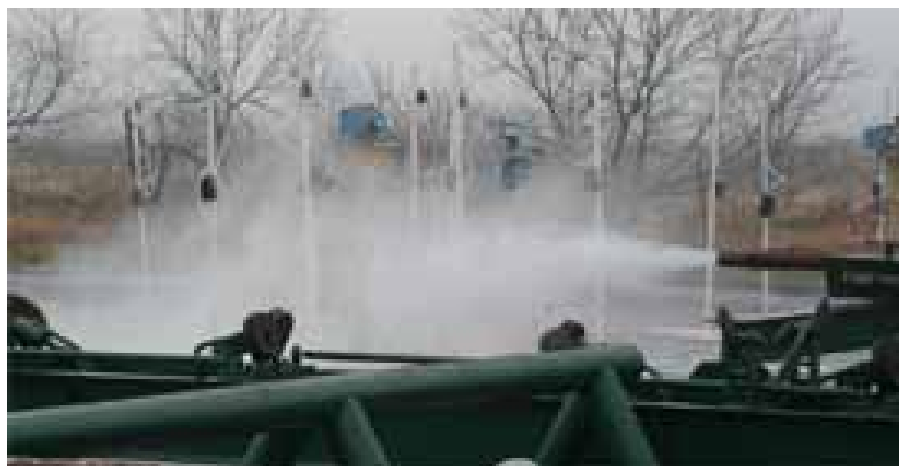
Fig 6 – Descaling process with scale being ejected by rattling machine
