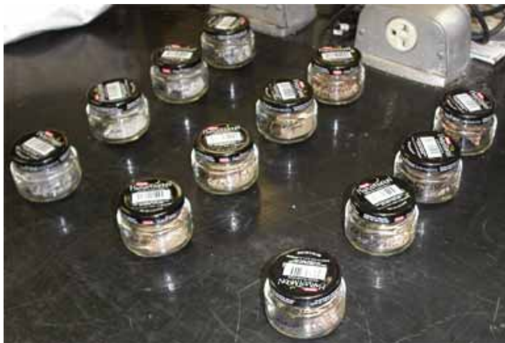
Fig 7 - Scale samples sealed for equilibration
