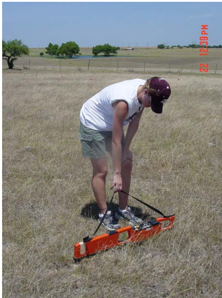
Fig. 1. The EM38 produced by Geonics Limited (Ontario, Canada). The unit is demonstrated in the vertical dipole position.
