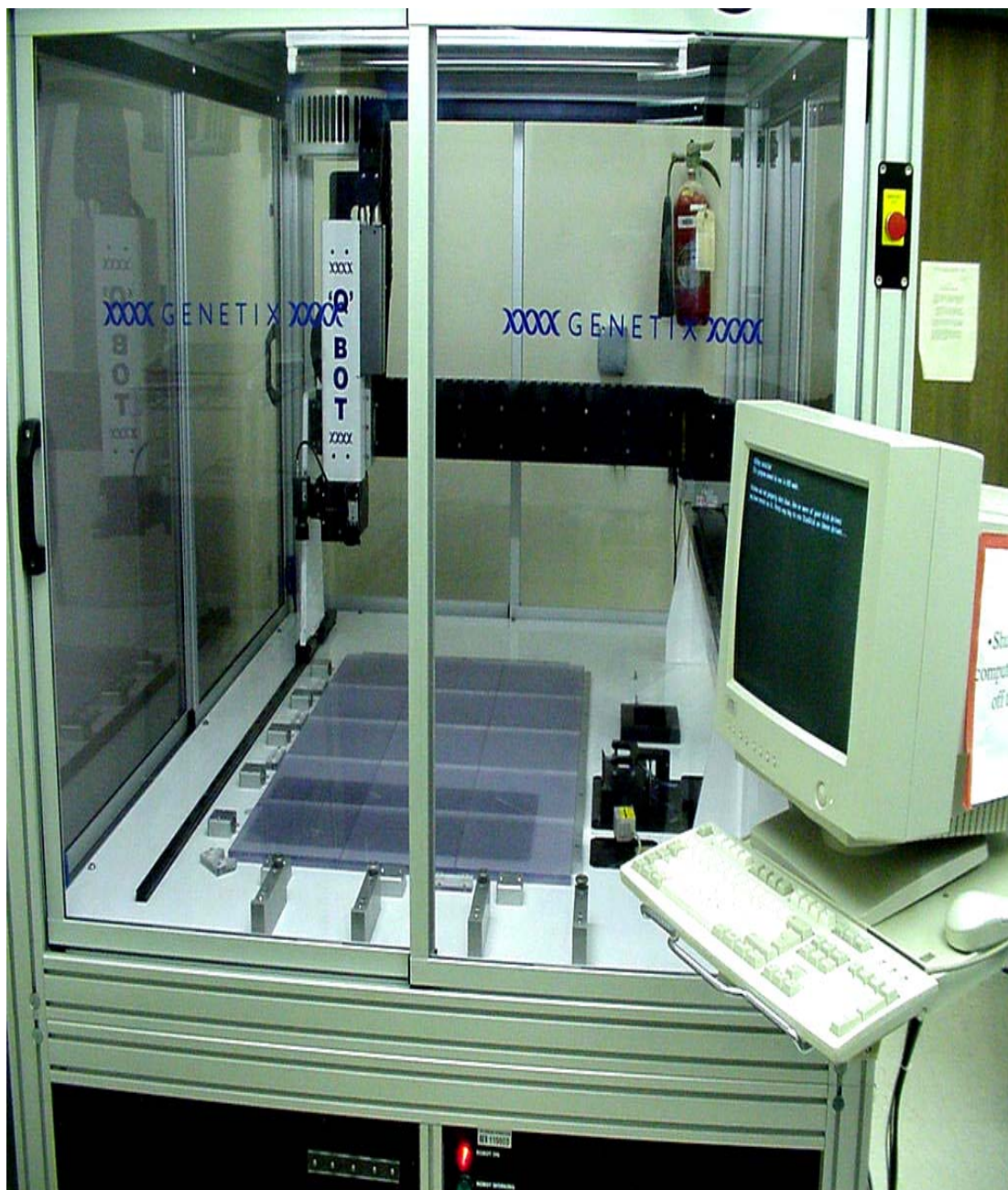
Fig. 5.2: Q bot robotics system. The system is capable of picking up to 3500 colonies/hour and inoculates them into either 96 or 384 well plates. The system has a CCD camera through which it picks the colonies and also is capable of gridding the colonies from 96 or 384 well plates onto large (22.2 X 22.2 cm) nylon membrane sheets.
