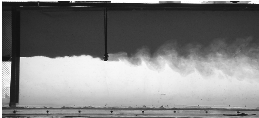
Figure 3. Visualization of the wake behind a cylinder with no buoyancy for a cylinder diameter of 1.6 cm and free steam velocity of 4 cm/s.
