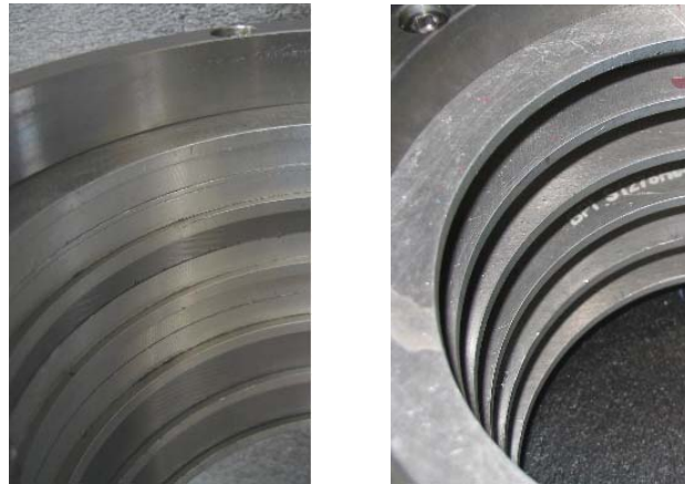
Figure 7.6 Six-bladed labyrinth seals with shallow (left) and deep (right) cavities
