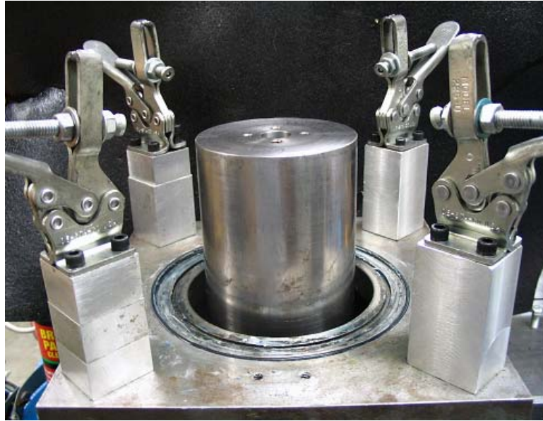
Figure 7.8 Non-rotating test-rig (seal not installed)
