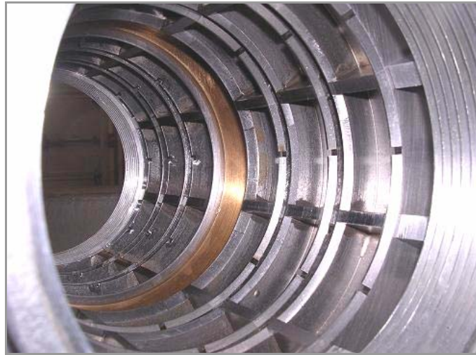
Figure 8.4 Ertas's 6-bladed pocket damper seal with beveled blades
