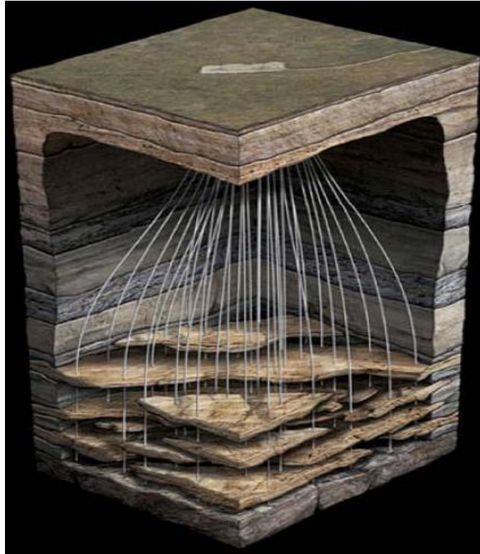
Fig. 34—Directional S-shape drilling in Pinedale field, Wyoming (Shell 2005).
