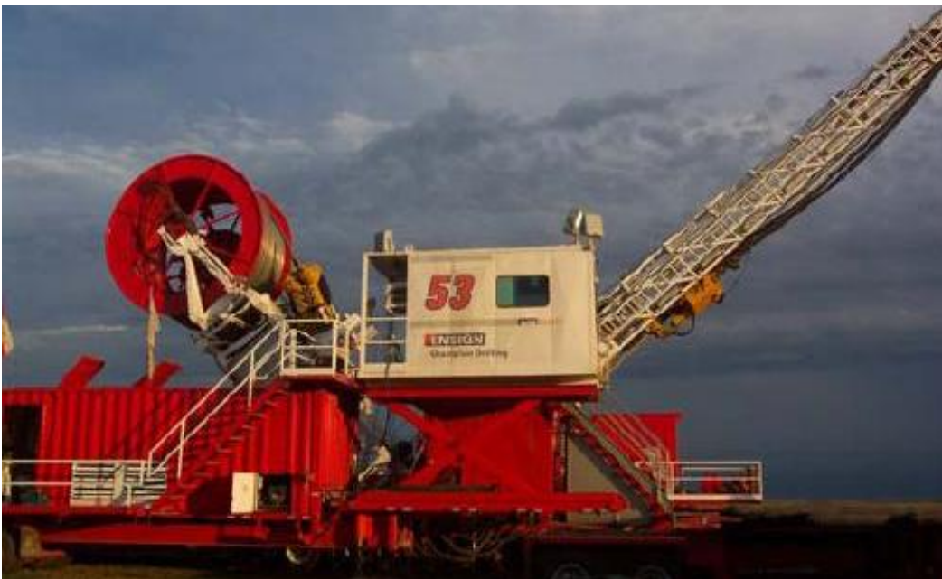
Fig. 15—Hybrid coiled tubing rig moving from conventional drilling to coiled tubing drilling (Shafer 2007).
