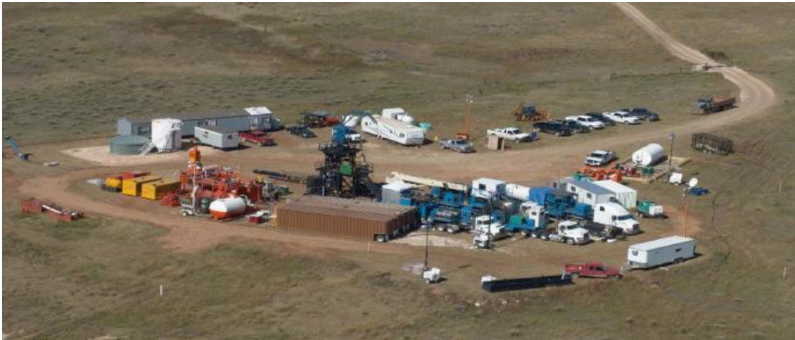
Fig. 28—Underbalanced drilling operation conducted in the Cleveland sands, Anadarko Basin (BP 2005).
