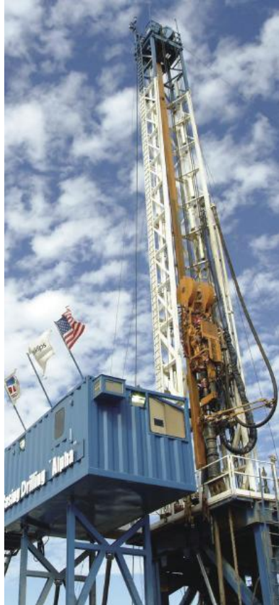
Fig. 17—Specially designed casing drilling rig (Tesco 2008).
