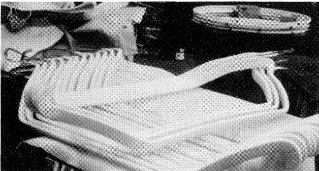
Figure 20. Taped and Formed Stator Coils Prior to Installing in Stator Core.
