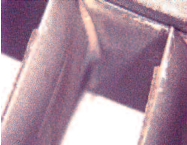
Figure 4 Salt deposits at the leading edge of the second-stage stator vanes (at 6.5x magnification). Hub is up in this image.
