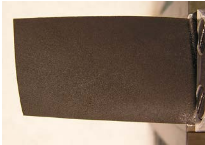
Figure 26. Blade Sprayed with Dirt/Tap Water Mixture in Heated Air Stream
