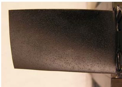
Figure 28. Blade Sprayed with Dirt/Commercial Detergent Mixture in Heated Air Stream
