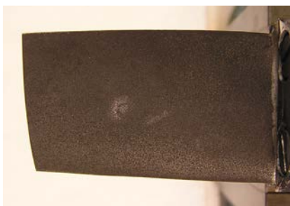
Figure 29. Blade Sprayed with Dirt/Gain/Deionized Water Mixture in Heated Air Stream
