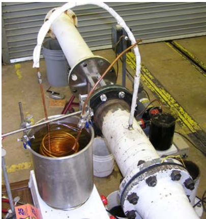
Figure 31. Heated Dirt/Water Injection Setup
