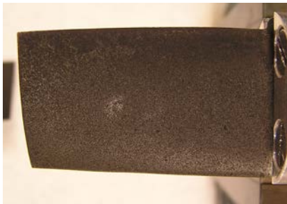
Figure 27. Blade Sprayed with Dirt/High-Purity Deionized Water Mixture in Heated Air Stream
