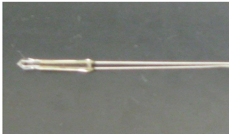
Figure 8: NTC thermistor code FP07DB104N supplied by GE Thermometrics Inc.
