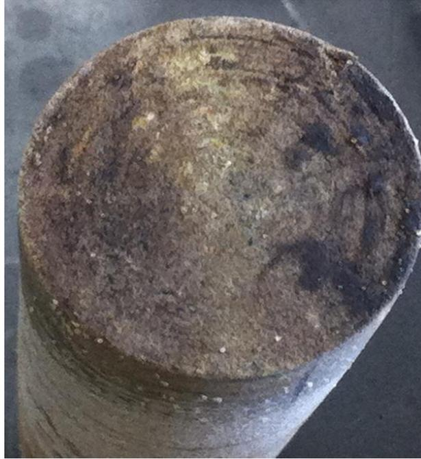
**Figure 57—Black precipitates on the inlet surface of sandstone core**
