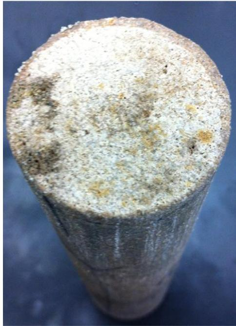
Figure 55—Grey precipitates on the inlet surface of carbonate core
