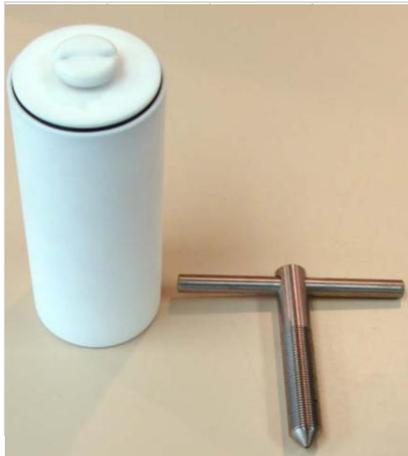
Fig. 14—Teflon liner with a T-screw
