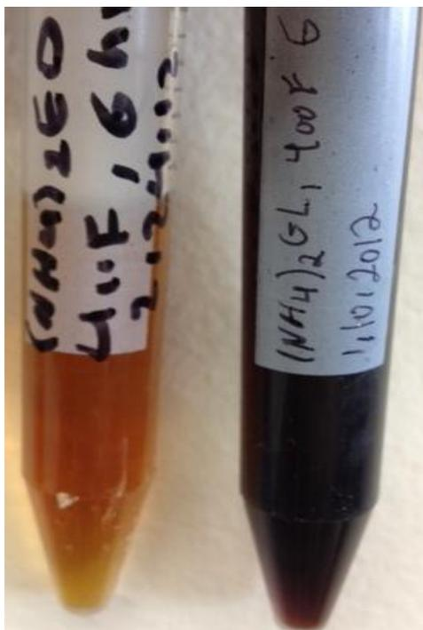
**Figure 38—Black precipitates dispersed in the solution of  $(\text{NH}_4)_2\text{GLDA}$  after heating at  $400^\circ\text{F}$  for 6 hours**
