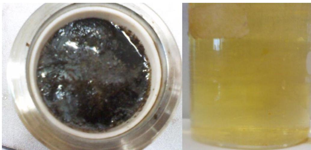
**Figure 23—  $\text{NH}_4\text{GLDA}$  after heating at  $400^\circ\text{F}$  for 6 hours and before heating**
