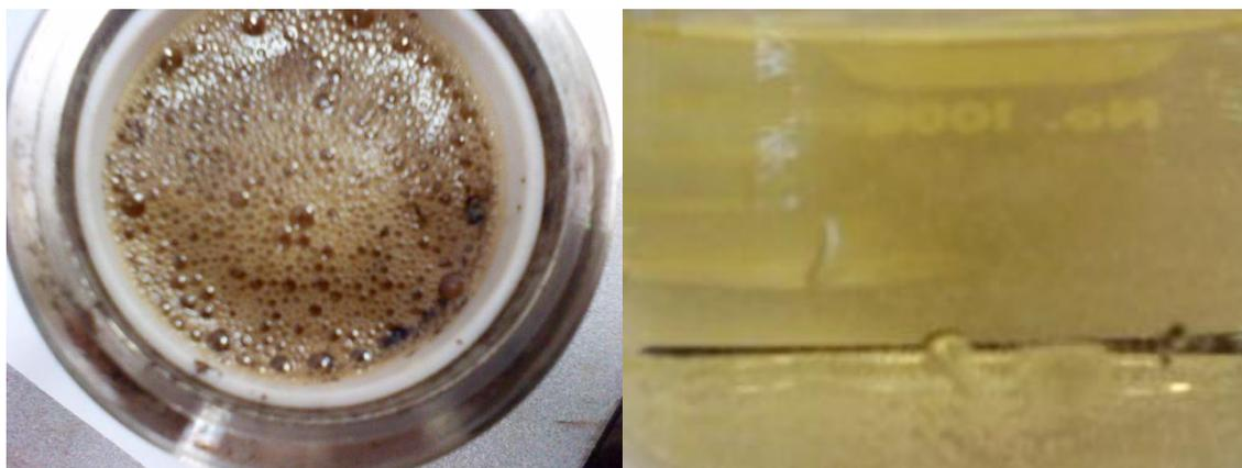
**Figure 24—  $\text{NaKGLDA}$  after heating at  $400^\circ\text{F}$  for 6 hours and before heating**
