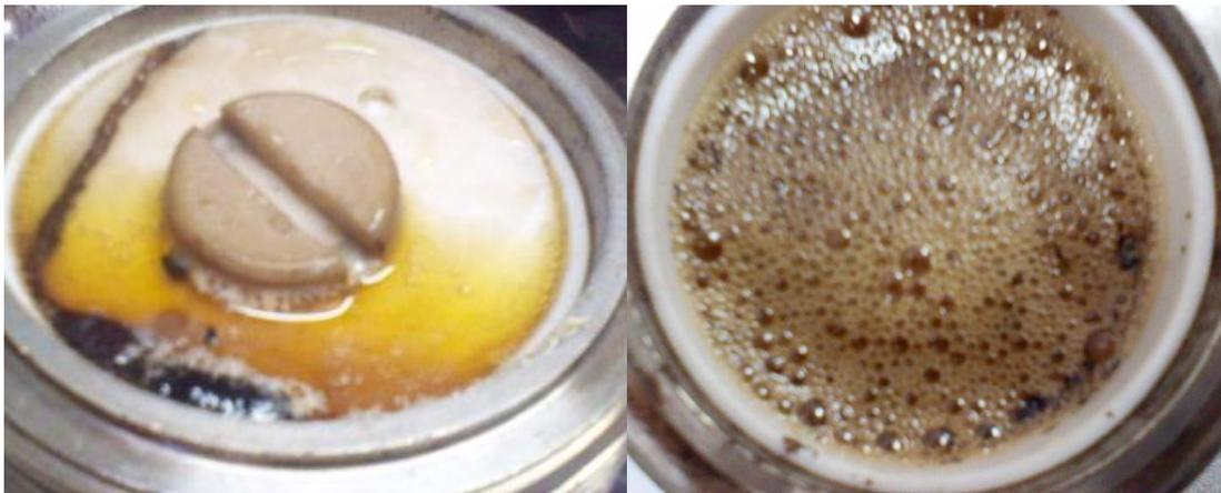
Figure 25— NaHEDTA after heating at 400°F for 12 hours and before heating
