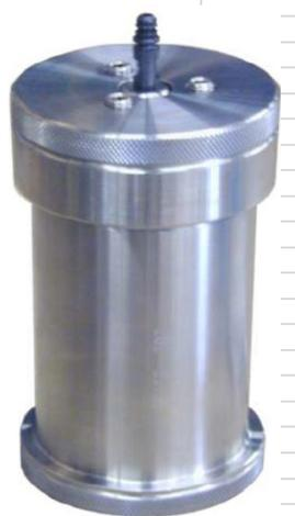
Fig. 13—Steel aging cell
